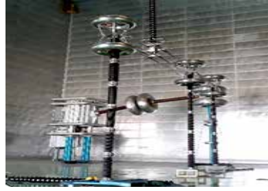
765 kV Porcelain Disc Single suspension insulator string under test
